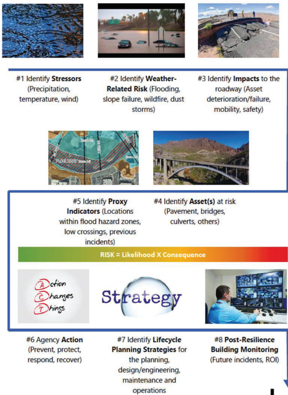
Figure 31. Life cycle Planning Template Process to Link Extreme Weather Climate Adaptation, Asset Management, and Infrastructure Resilience 5
