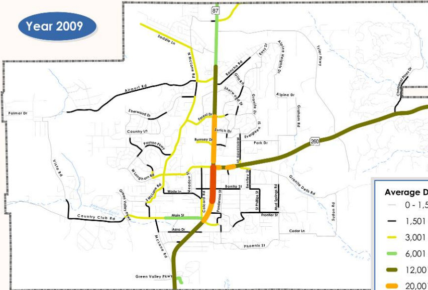
Year 2009 traffic volume estimates are based on existing roadway conditions with existing population and employment growth conditions.
