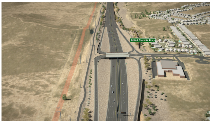
Simulation of the half Diverging Diamond Interchange at Desert Foothills Parkway (Image courtesy of ADOT)
