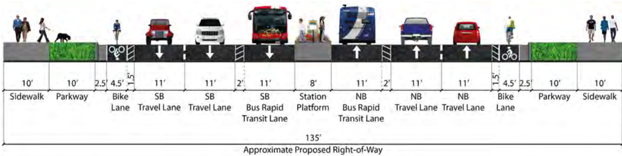
Figure 5-6: System Alternative 13 Cross Section at Platform Locations
