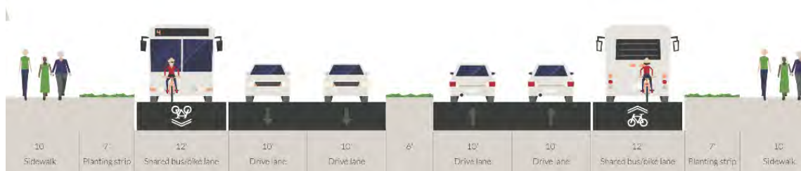
Figure 4-4: System Alternative 12 Mid-Block Cross Section
