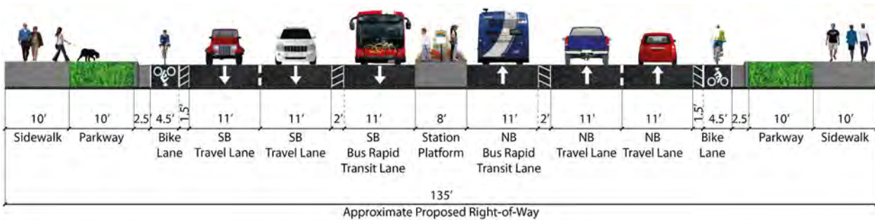
Figure 4-13: System Alternative 13 Cross Section at Platform Locations
