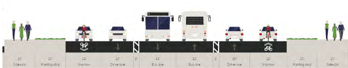
Figure 4-5: System Alternative 13 Mid-Block Cross Section
