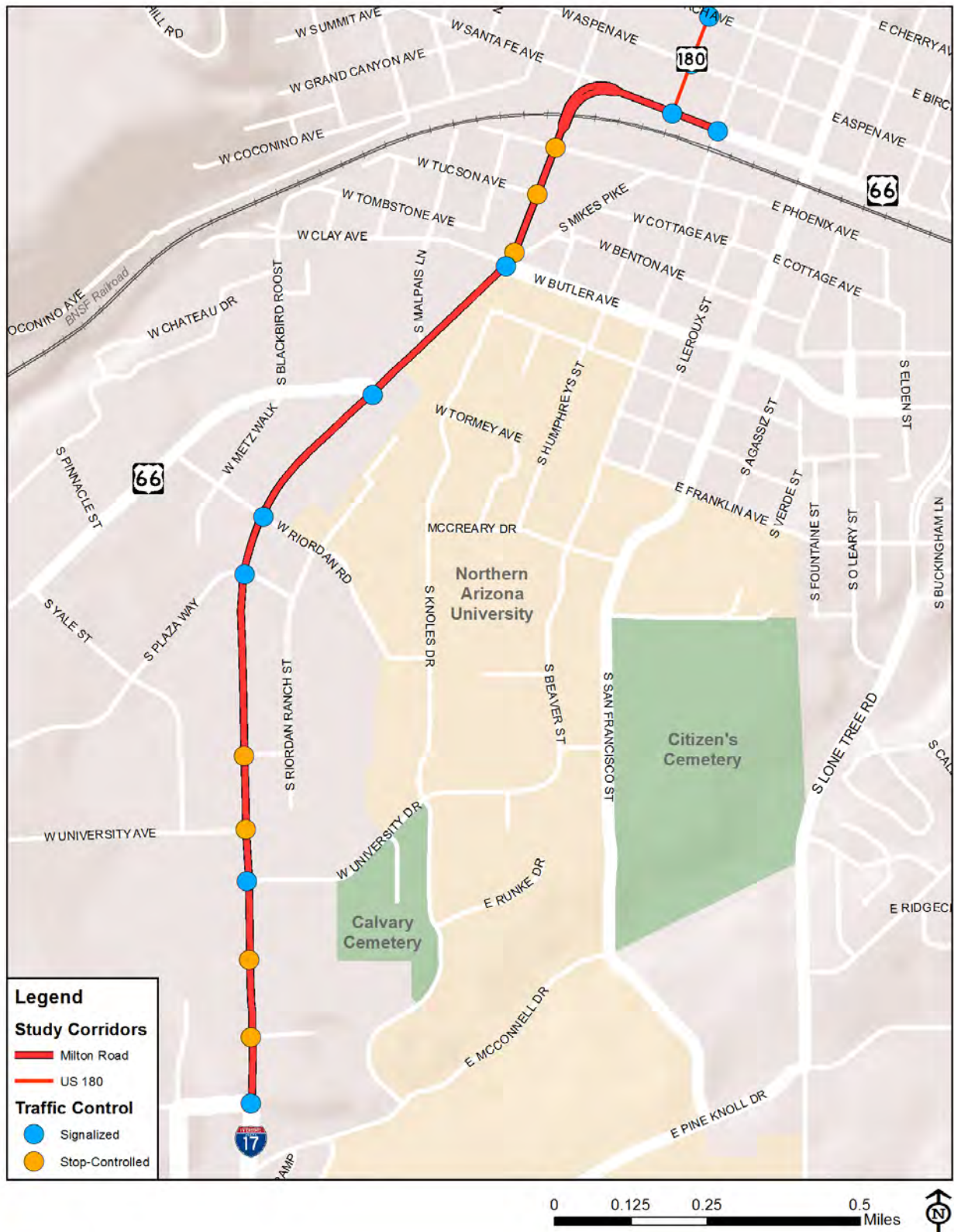
Figure 5-5: Existing Traffic Control at Study Intersections
